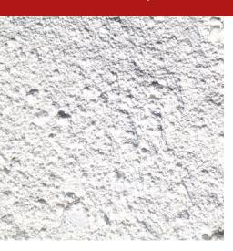
Natural hydraulic lime, white coloured, obtained through firing, in a vertical oven in refractory stone and bricks, at temperatures of 1100°C, of constant quality select marly limestones, specific for mortars, plasters and substrate screeds in ecological building works and in interventions of historical and monument restoration.
