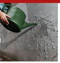
Nano-dispersion of water-based reactive amino functional silanes and siloxanes. Water-repellent impregnating agent, colourless, non-filming, protects plasters, cementitious systems, natural stones, tuff, etc., from adverse weather conditions, frost and thaw cycles and from atmospheric aggressions. It does not alter the colour of the surface and does not change the original appearance and breathability.
