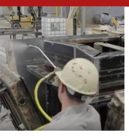
Release agent based on selected organic compounds, promoting removal and anti-corrosive agents, ready-to-use, specific for metal moulds. Distak-M should be used undiluted, sprayed directly on the surfaces to be treated.
