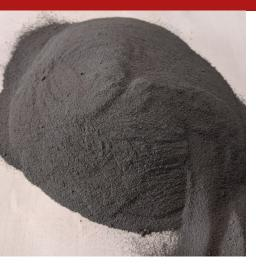
Selected grey silica fume for the production of high density and high performance conglomerates (waterproofness, chemical stability, mechanical strength etc.), for packaging sulphate-resistant, anti-leaching mortars, plasters, grouts and concretes.
