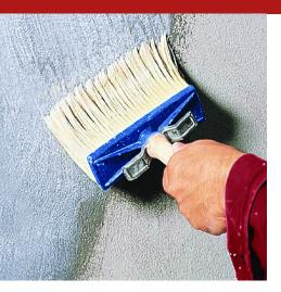
Water-based anti-condensing wall covering, with excellent fixing and anchoring properties, with good coverage based on high penetration acrylic resins, 3M Glass Bubble, pigments, fillers and covering fillers. Suitable as an anti-condensation fixative primer, prior to painting or coating the plaster with anti-condensation paints or plasters (-THERM).
