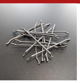
"Carbon steel fibres, obtained by the cutting of metal wire, with improved adhesion profile, for three-dimensional general structural reinforcement of cement-based conglomerates. The addition of Readymesh MF-500 significantly increases the mechanical performance of the structure in terms of toughness, ductility, fatigue, dynamic stress, shock, wear, tensile and shear strength and even post-cracking and damage behaviour."
