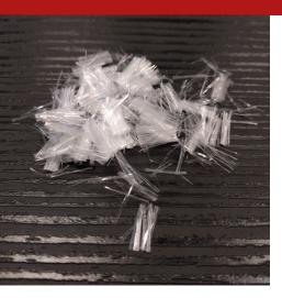
Readymesh PW-120 is an auxiliary fibrillated polypropylene micro-fibre, with a length of 12 mm, suitable for adding concrete in general. The addition of Readymesh PW-120 to the mixture allows for preventing the phenomenon of cracking from plastic shrinkage of the concrete, as well as having positive effects as regards the ductility of the mixture, the resistance to freezing/thawing, the shock resistance and overall watertightness.
